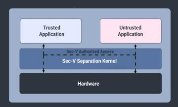
The Sec-V separation kernel architecture recognizes that VMs hosted in isolation with a secure communication channel can cater to multiple industry segments. Therefore from ground up the design of the hypervisor is focused on being capable of serving these various segments with as much commonality as possible.
